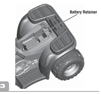
Carefully lower the battery into the battery compartment.
